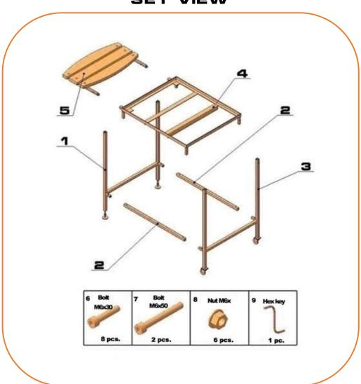
The assembly process comprises of 4 stages and the table can be assembled by one-man. The table shall be assembled exactly according to the scheme presented below. The assembled parts are shown in gray. The parts are to be assembled are shown in orange.
